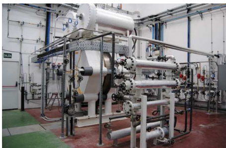
IHT Electrolyser – FHA facilities (10 Nm 3 /h H 2 )
